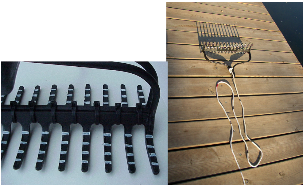
Figure 1: Double-headed rake for aquatic vegetation sampling
